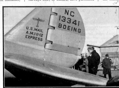
The massive rudder of the Boeing 247-D, an American 10-seater twin-engined monoplane.
