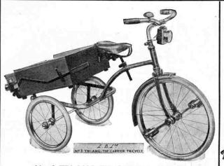
No. 3 TRI-ANG TIP CARRIER CYCLE New Model with CHROMIUM-PLATED fittings. Strongly made of best weldless steel cycle tubing, ball bearings throughout, leather saddle, tangent spoke wheels, jointless sponge tyres. Fitted with box at rear and special tipping gear. Frame blue. Handlebars, forks, etc., CHROMIUM PLATED. Box finished red. Price 79/6
