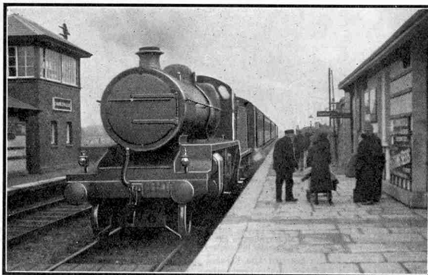
A typical Irish station scene showing an up train from Cork at Charleville. The locomotive is No. 398, assembled from parts made at Woolwich, and fitted with driving wheels 6 ft. 1 in. in diameter. Photograph by A. G. Beatt, Athboy. In the upper photograph on this page is G.S.R. No. 500, the first of the modern 4-6-0 mixed traffic locomotives constructed at Inchicore Works. It is used on main line trains between Dublin and Cork. Photograph by courtesy of the Great Southern Railways.
