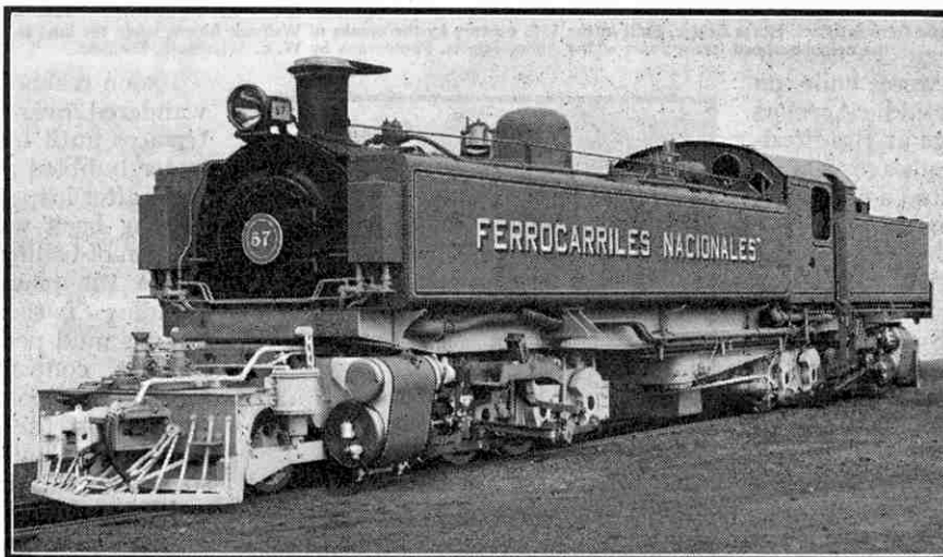
One of the powerful 2-8-0+0-8-2 Kitson-Meyer locomotives recently built for the National Railways of Colombia. Illustration by courtesy of Robert Stephenson & Co. Ltd., Darlington.
