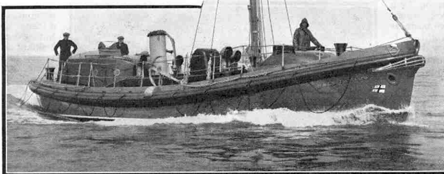
Barnett Stromness type life-boat 51 ft. long, driven by two 60 h.p. engines.
