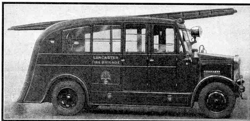
A streamlined fire engine owned by the Lancaster Corporation. It has a 65 b.h.p. petrol engine, "Hatfield" pump and an extending ladder, which is carried in a trough in the roof of the body.
