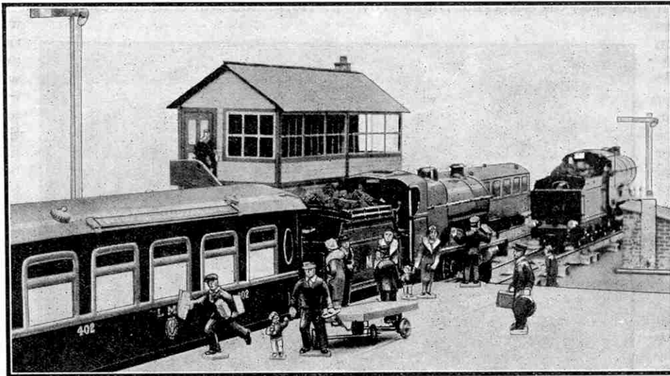
A long-distance train made up of Hornby No. 2 Saloon Coaches. As the load is a heavy one a pilot engine is backing down to assist the train engine that is already coupled up.
