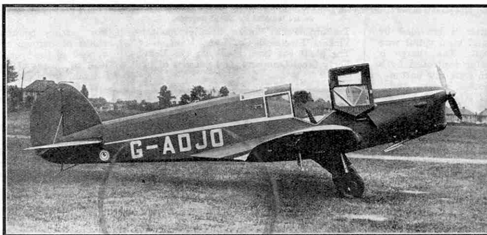
The B.A. "Eagle" low wing monoplane. The doors meet over the centre of the cabin, and when both are open, as shown, there is unrestricted access and exit on each side of the cabin. This aeroplane is an improved version of the British Klemm "Eagle." This illustration and the upper one on the opposite page are reproduced by courtesy of "The Aeroplane."
