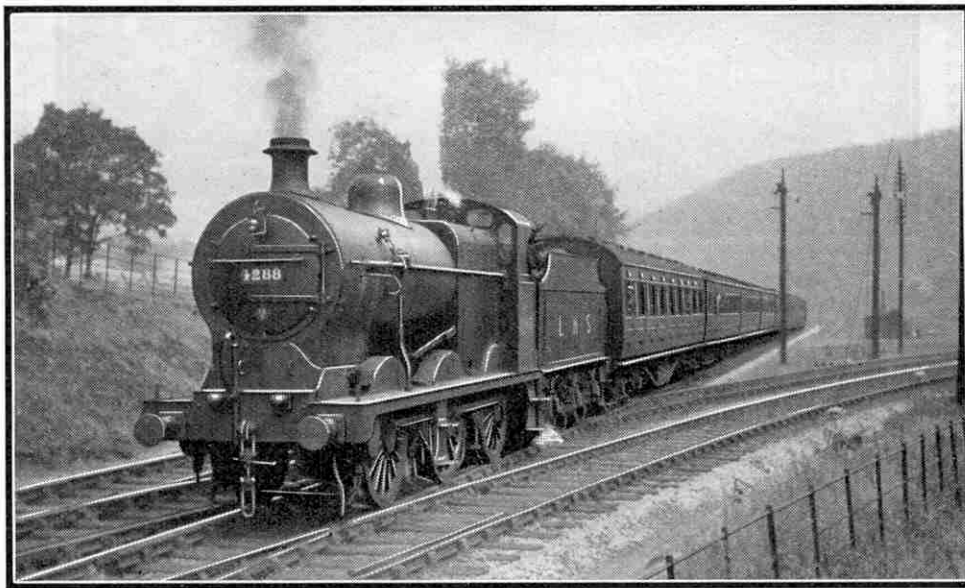
An L.M.S.R. local train hauled by the 0-6-0 Standard freight locomotive No. 4288. When required these engines do useful work on the slower passenger and excursion trains. (H.R.C. Prize-winning photograph.)
