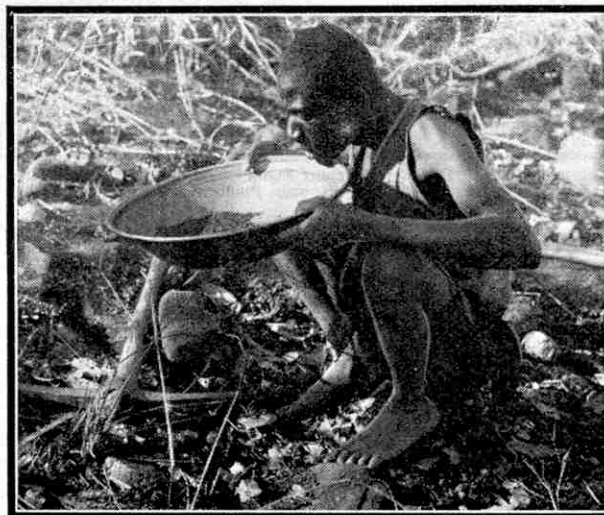
Dry blowing for gold. The gravel is pounded in a pan, shaken and swirled round, and the lighter waste matter is blown away.
