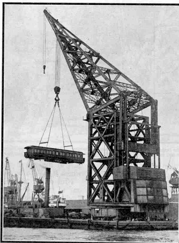
The 150-ton floating crane "London Mammoth" engaged on the shipment of railway coaches for South Africa. Photograph by courtesy of the Port of London Authority.
