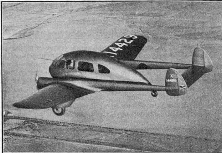
The American "Crusader," a novel type of low wing monoplane in which the tail unit is mounted at the end of long, tubular booms. Photograph reproduced by courtesy of "Les Ailes," France.
