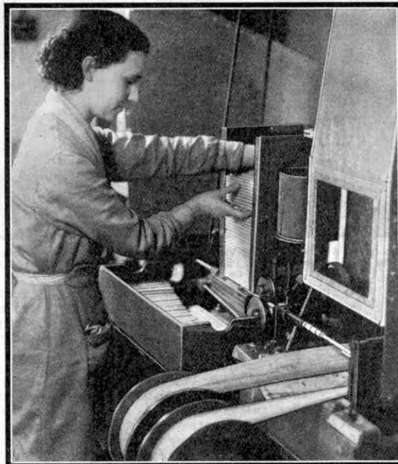
Painting machine hopper for pencils, which are automatically coated with cellulose paint and dropped on a travelling belt to dry.
