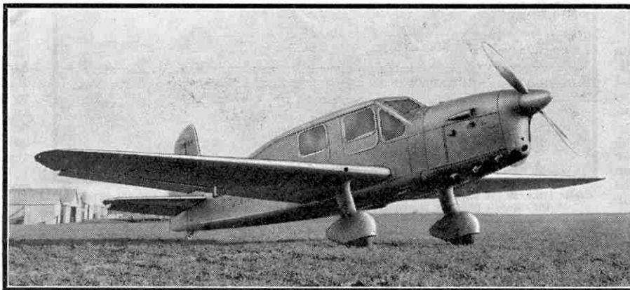
The "Simoun" Caudron low wing monoplane. The curved roof of the cabin gives the machine a humped appearance.
