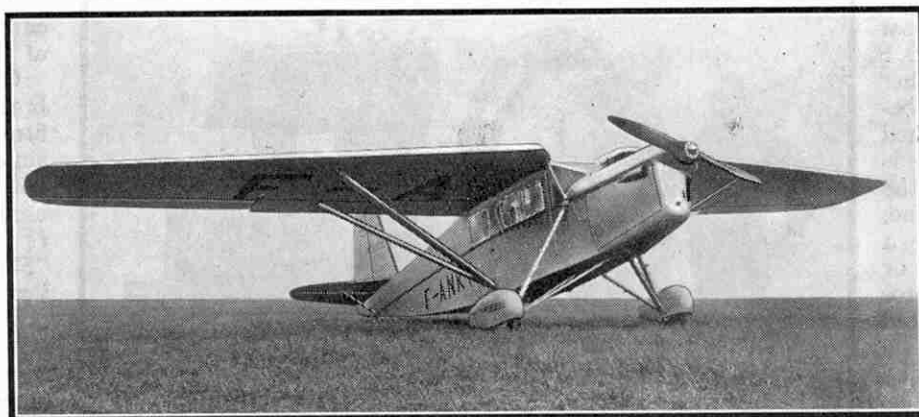
One of the few types of high wing monoplanes made by the company is the "Fregate," shown above. It is a cabin machine with seating for three passengers.
