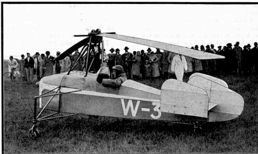
The "direct-lifting" Autogiro built by G. and J. Weir, Ltd., Glasgow. It can rise straight up into the air to a height of 25 ft. to 30 ft. The illustrations to this article are by courtesy of the Cierva Autogiro Co., Ltd.
