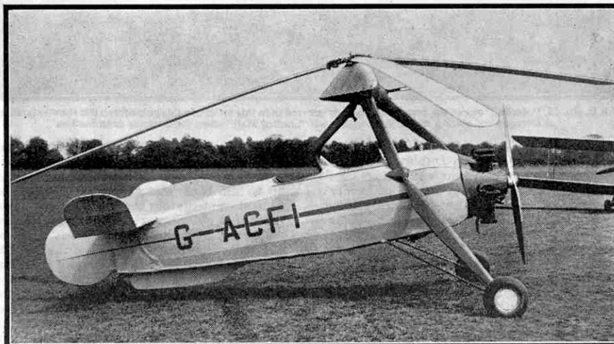
The C.30 "direct control" Autogiro, which requires a short forward run when taking off, but can descend vertically.
