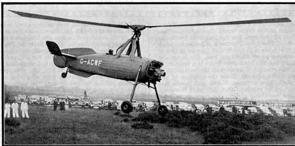
A C.30 Autogiro, converted to "direct-lifting," taking off without any forward run.
