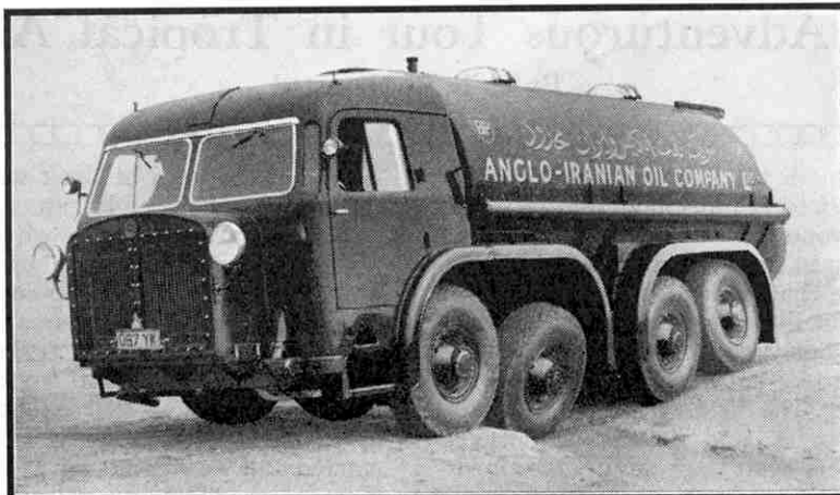
Flexibly mounted road wheels to facilitate passage over rough surfaces are an important feature of this giant petrol tank lorry, which has been built for service in the Iranian Oilfields. Photograph by courtesy of Straussler Mechanization Ltd.
