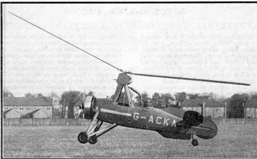
The Cierva C.30 "Direct-control" Autogiro descending vertically. This machine has long rotor blades and can take off after only a short run along the ground. Photograph by courtesy of Cierva Autogiro Co. Ltd.
