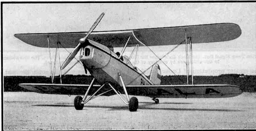
The Koolhoven F.K.46, a Dutch two-seater training biplane with staggered wings. It is fitted with a 130 h.p. D.H. "Gipsy Major" engine and has a top speed of 108.6 m.p.h. Photograph reproduced by courtesy of N. V. Koolhoven Vliegtuigen, Rotterdam.
