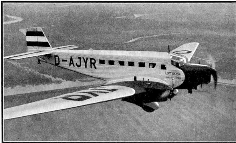
A Junkers Ju.52/3m seen from another aeroplane flying slightly ahead of it. This triple-engined monoplane carries up to 17 passengers, and can be adapted for use as an air ambulance.
