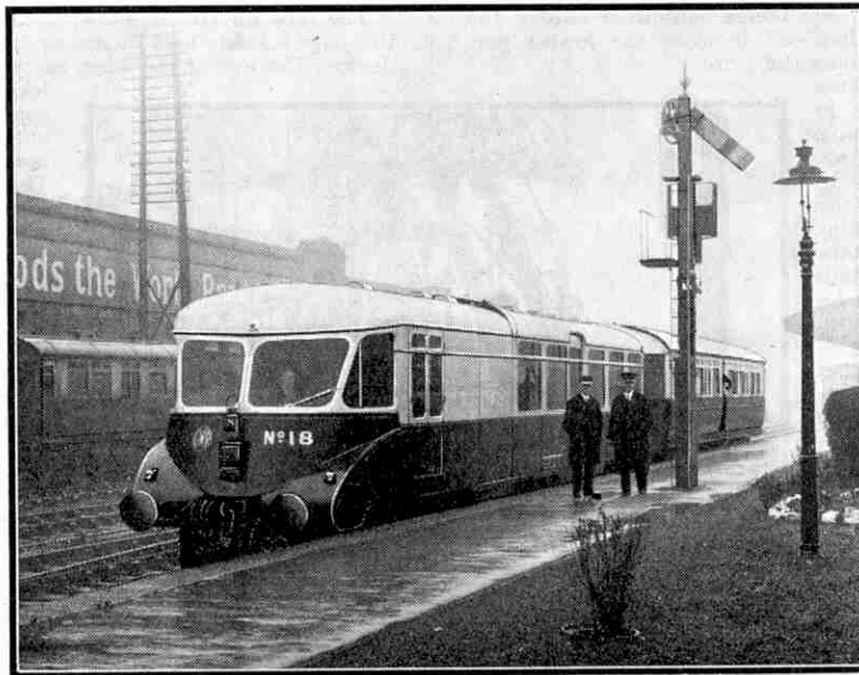
"No. 18," the latest A.E.C. oil-engined railcar on the G.W.R. It has been specially designed to haul a trailer coach or other vehicles in branch line operation. Photograph reproduced by courtesy of The Associated Equipment Co. Ltd., of Southall, the builders of the vehicle.
