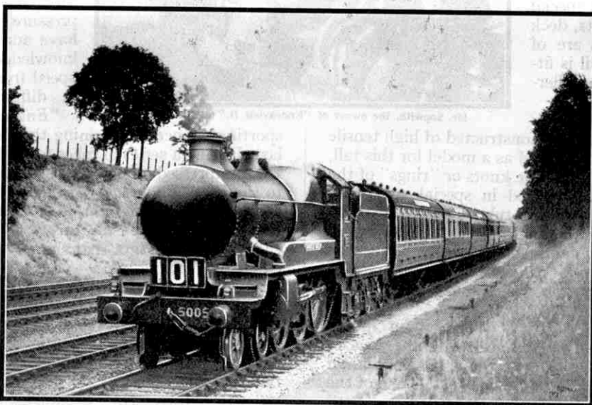
G.W.R. 4-6-0 locomotive " Manorbier Castle ," as modified to reduce wind resistance, on an excursion train. A feature of G.W.R. summer working is the system of numbers prominently displayed in front of the engine to assist the staff in identifying a particular train. Photograph by M. W. Earley, Reading.
