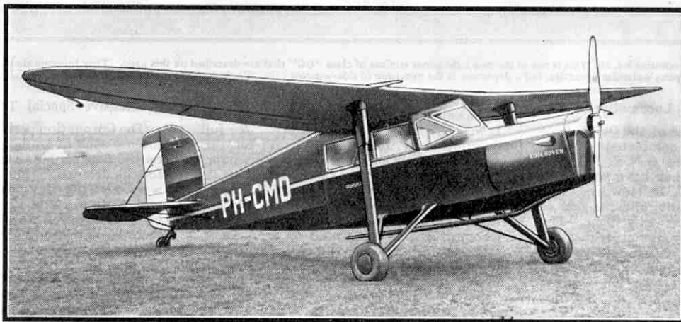
The FK 43 four-seater cabin monoplane in which the long telescopic legs of the undercarriage extend up to the wing. The illustrations to this article are reproduced by courtesy of N.V. Koolhoven Vlietuigen, Rotterdam.
