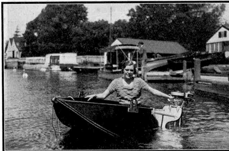
A 7 ft. 10 in. dinghy designed for use with a lightweight outboard motor. The motor is attached to a bracket on the port side. Photograph by courtesy of E. P. Barrus Ltd., London.
