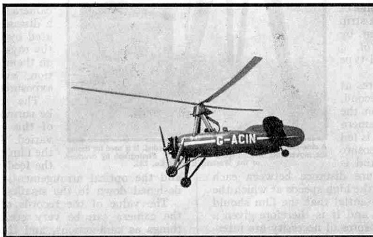
The Cierva C.30 Autogiro in the air. The great length of the rotor blades is very noticeable. This machine takes-off after a forward run of only a few yards, and can alight without a run. Photograph by courtesy of Cierva Autogiro Company Ltd.
