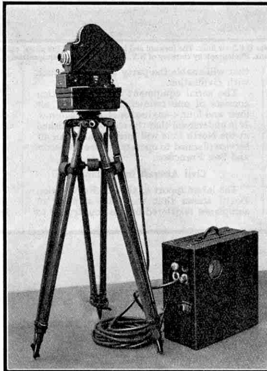
A cine-camera that takes 2,500 pictures a second. It is used for timing the movements of high-speed machinery. Photograph by courtesy of the Western Electric Co. Ltd.
