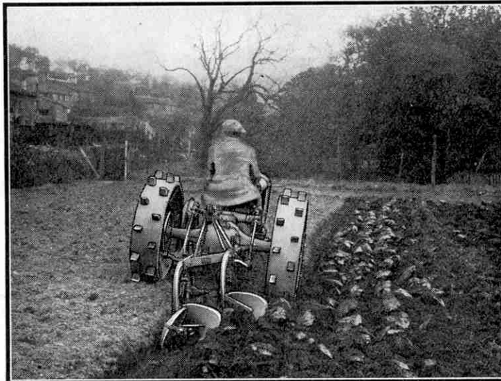
A Ferguson tractor hauling a double plough. A patent linkage and hydraulic control keep the plough level and at a constant depth in the soil. Photograph by courtesy of David Brown Tractors Ltd., Huddersfield.
