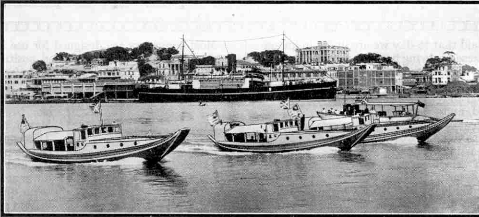
Chinese sampans in which Diesel engines have been installed. These vessels can turn almost in their own length when travelling at full speed. Photograph by courtesy of Ruston and Hornsby Ltd.
