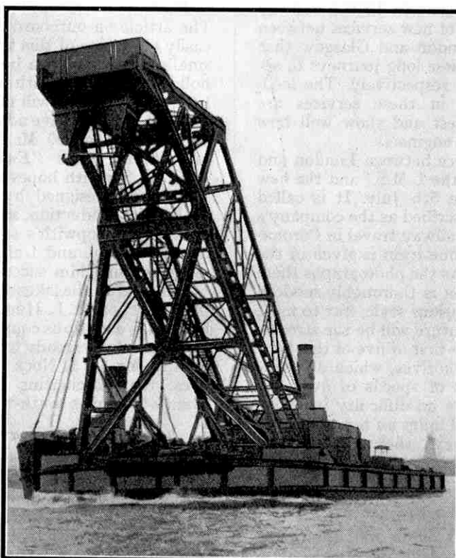
The floating crane "Gironde," which was specially built for handling the concrete piles used in the making of Le Verdon Harbour. For the illustrations to this article we are indebted to Werf Gusto, Firma A. F. Smulders, Schiedam, Holland.
