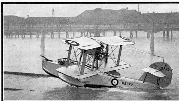
Another Vickers Supermarine aircraft, the "Walrus" single-engined amphibian. It is used by the Fleet Air Arm for reconnaissance duties.
