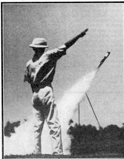
A small pilot rocket being fired in advance of the Coronation Rocket, so that the direction of the wind currents could be observed before firing the main rocket.
