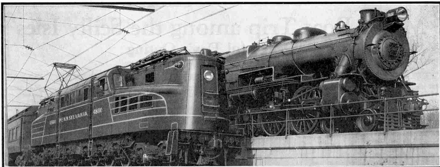
The new and the old forms of motive power on the Pennsylvania Railroad. On the left is one of the new streamlined electric locomotives of class GG-1 that were specially designed for hauling the fastest and heaviest expresses between New York and Washington. On the right is a 'Pacific' steam locomotive of class K4S.
