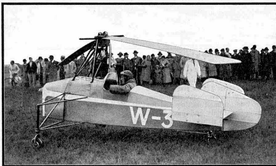
The "direct-lifting" Autogiro, which can rise straight up into the air and can descend vertically. Photograph by courtesy of the Cierva Autogiro Co. Ltd.
