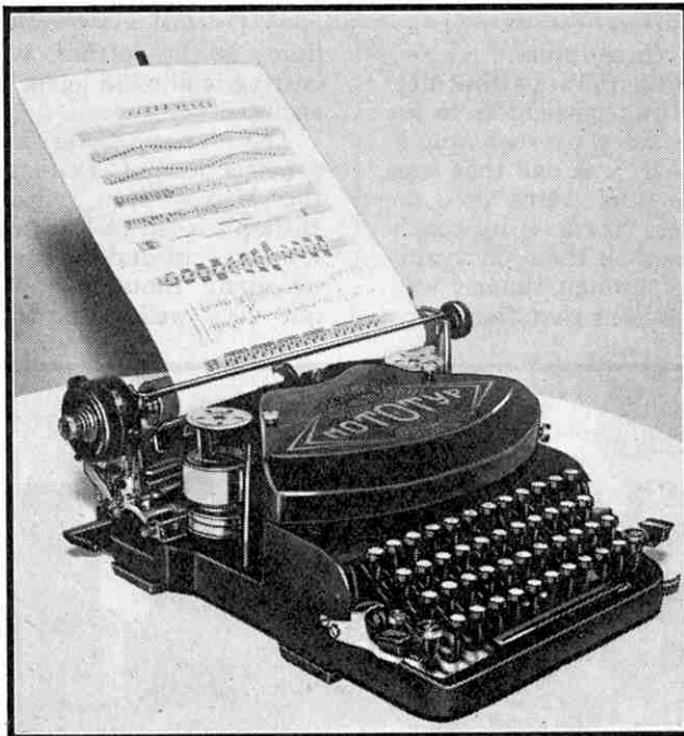
A music typewriter. With this machine, which is the work of a German inventor, a standard line of music can be written in from two to three minutes.
