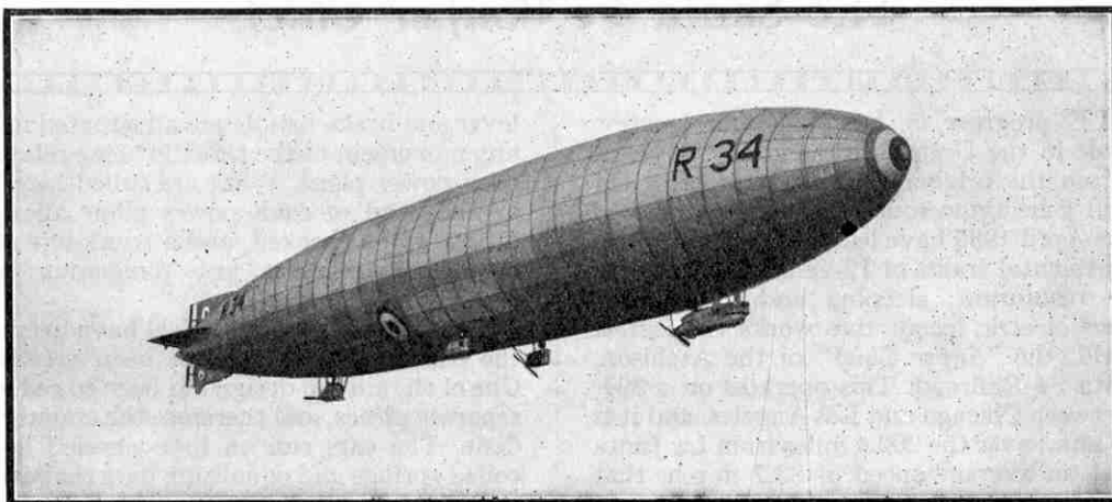
The British airship R.34 on a trial flight. In 1919 she flew across the Atlantic to America and back, and was the first airship to accomplish this feat. She was 643 ft. long, and had a top speed of 62 m.p.h.
