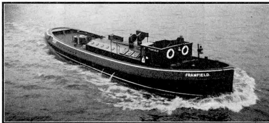
A tug without a funnel. A good example of a type with Diesel-electric propulsion.
