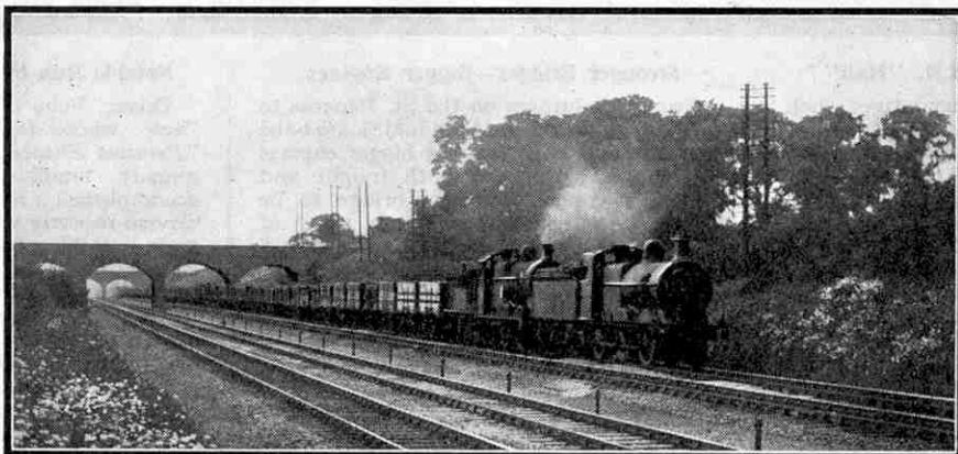
A coal train on the Midland route of the L.M.S. before the introduction of the "Beyer-Garratt" articulated locomotives, with two 0-6-0 engines at its head. The illustrations on this page are reproduced by courtesy of the L.M.S.
