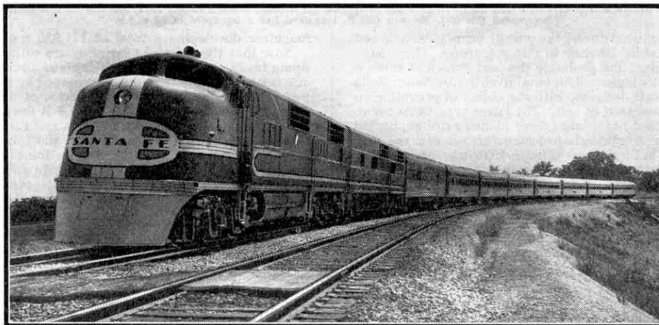
The "Super Chief," the fastest train in the world, hauled by a streamlined Diesel-electric locomotive of 3,600 h.p. Photograph by courtesy of the Atchison, Topeka and Santa Fé Railroad.
