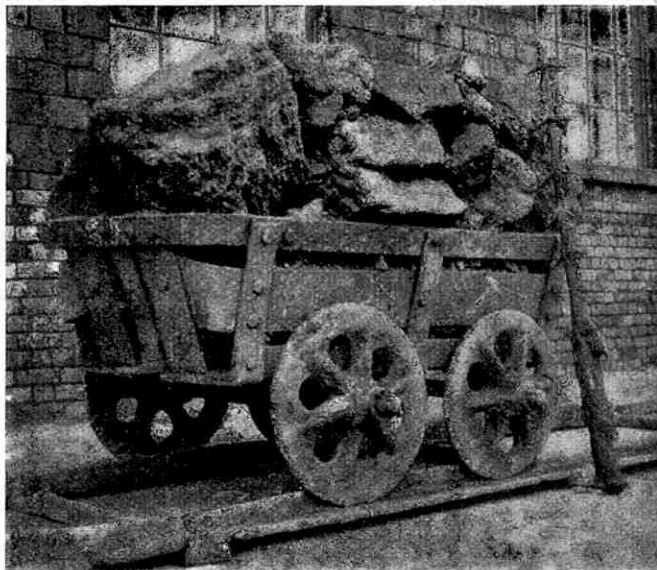
A loaded coal tram of the type used in South Wales 125 years ago for transporting iron ore. It is now in the National Museum of Wales.
