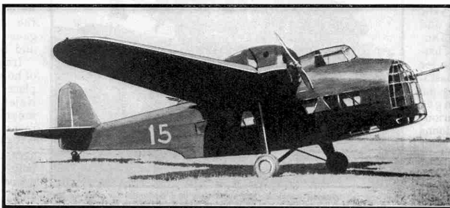
Broadside view of the FK 50B, a twin-engined long range bomber. It is armed with three machine guns, one of which occupies the gun turret in the nose of the fuselage.
