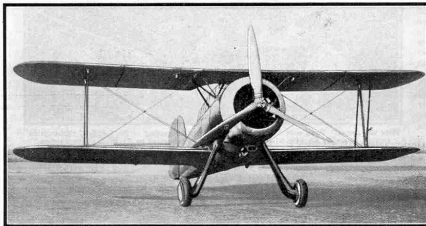
The Koolhoven FK 52 two-seater general purpose fighter. The two cockpits are under one roof so that the pilot and gunner can talk to each other without difficulty.
