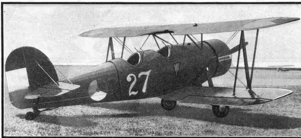
The FK 51 trainer, which can be used for instruction, aerobatics, radio operation, bombing and aerial photography.
