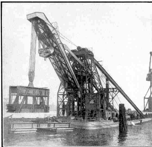
A giant floating crane for the Manchester Ship Canal. It can lift loads up to 250 tons and will be described in an article in next month's issue. Photograph by courtesy of Werf Gusto Ltd. (Firma A.F. Smulders) Schiedam, Holland.
