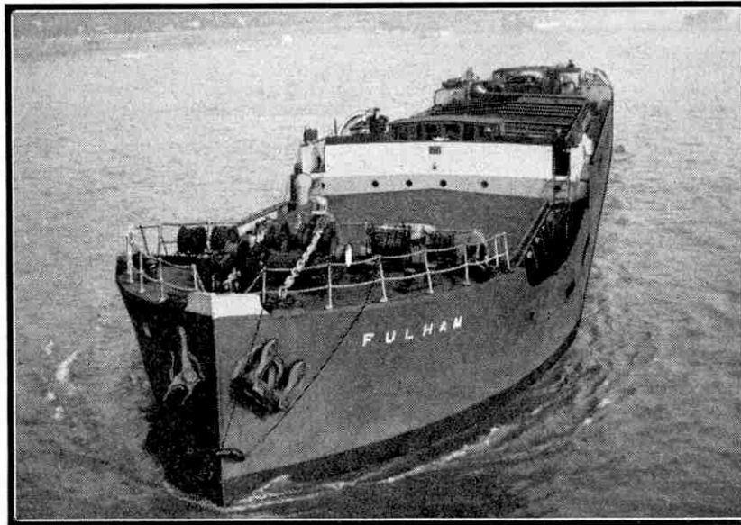
The steam collier "Fulham," owned by the Fulham Borough Council, inward bound at Battersea Reach. The vessel in this illustration, and that in the upper one on the opposite page have their funnels lowered to enable them to pass under bridges.
