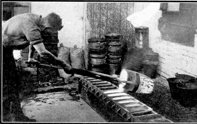
Molten gun metal from a 150-lb. "Carborundum" crucible being poured into ingot moulds. The caster pours the metal and at the same time holds back oxides and dross.
