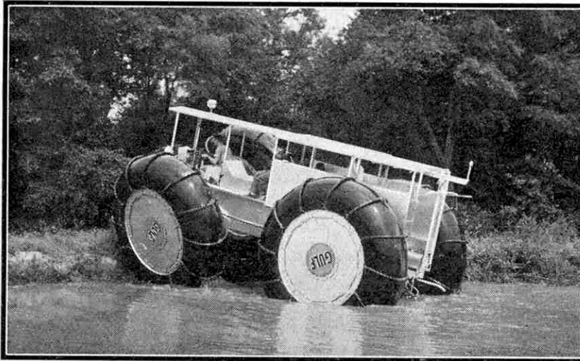
The marsh buggy climbing on to the bank of a muddy stream with the aid of the treads on its huge tyres. We are indebted to the courtesy of the Gulf Oil Corporation, Pittsburgh, U.S.A., for this illustration, and for the photograph on which our cover is based.
