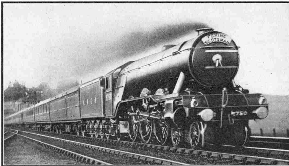
A Gresley "Super-Pacific," No. 2750 "Papyrus," hauling "The Flying Scotsman." In March 1935, in the course of a high-speed non-stop test run, this locomotive reached a maximum of 108 m.p.h., then a British record.
