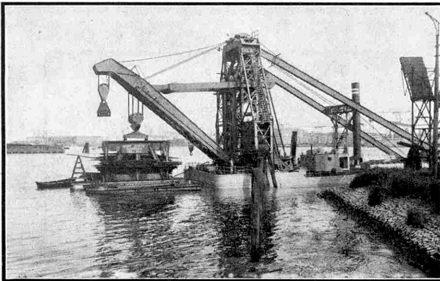
The 250-ton floating crane built for the Manchester Ship Canal Company, and described on this page. In the illustration the jib is shown in position for carrying out salvage work. We are indebted for our photograph to Werf Gusto Ltd. (Firma A. F. Smulders), Schiedam, Holland.
