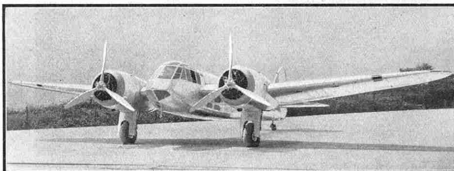
This view shows the "Blenheim" to be a monoplane of the middle wing type, a wing arrangement that is becoming increasingly popular for military aircraft. Photograph reproduced by courtesy of the Bristol Aeroplane Co. Ltd.
