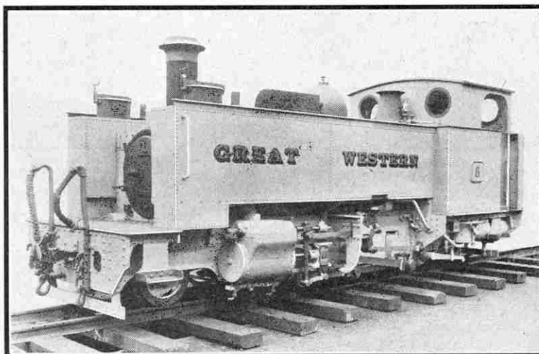
A diminutive G.W.R. tank locomotive. This little engine is in service on the Vale of Rheidol line, a narrow gauge branch from Aberystwyth to Devil's Bridge. Photograph by courtesy of the G.W.R.
