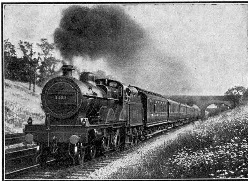
L.M.S. Standard Compound No. 1100 on a heavy down express. This photograph was taken some years ago when experiments were being made with oil firing. This accounts for the round tank on the tender.
