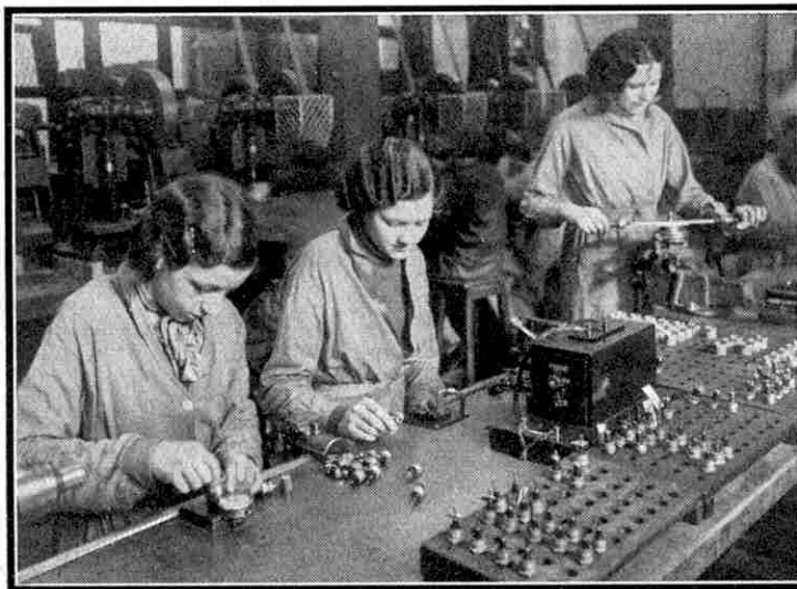
Assembling and testing plugs. In the centre these are seen undergoing high voltage trials, and on the left they are being examined to make sure that the electrodes are central.
