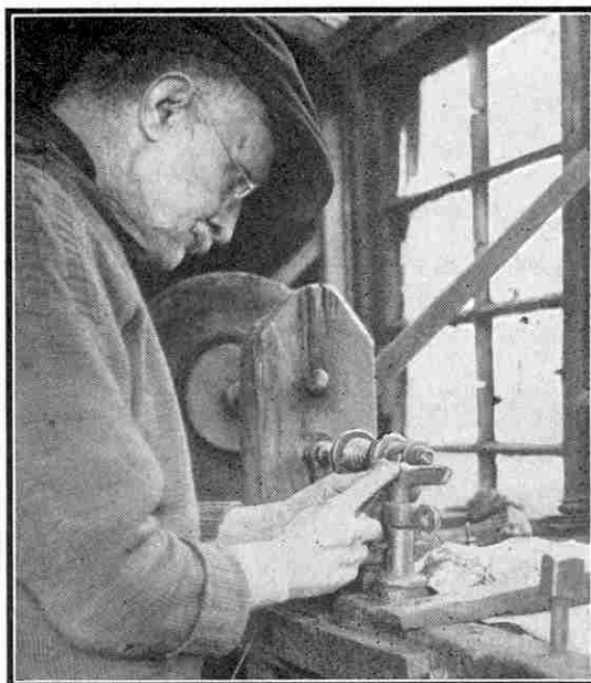
A Whitby jet worker at his primitive treadle lathe. The tiny flat pieces of jet are ground and polished twice, the final polishing with sheepskin giving a perfect surface.
