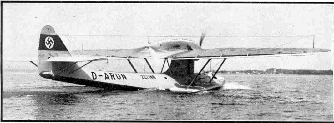
"Zephyr," one of two Dornier Do. 18E flying boats used by Deutsche Luft Hansa in experimental flights across the North Atlantic in 1936. This improved type has succeeded the "Wal" on the company's South Atlantic service.
