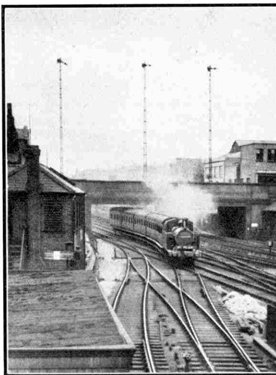
An L.M.S. standard 0-6-0 tank locomotive on a local train at Dalston Junction. The unusually tall signals are an outstanding landmark at this point. Photograph by W. S. Garth, Preston.
