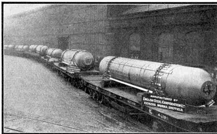
Nine completed forged boiler drums, manufactured as explained in this article, leaving the works of the English Steel Corporation for Australia.
