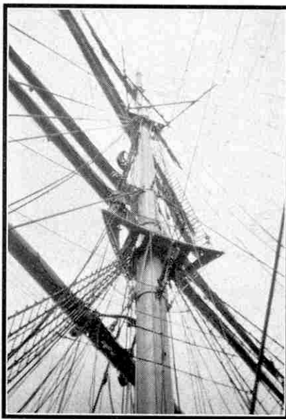
Part of the rigging of the "Viking," showing the "lubber's hole" at the top of the lower mast. Photograph by W. F. Fry, Gloucester.
