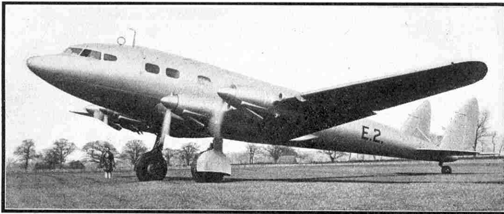
The D.H. "Albatross" long-range monoplane. Since the photograph was taken this aeroplane has been fitted with a wider tail unit. A fleet of air liners of this type will be put into service by Imperial Airways this summer.
