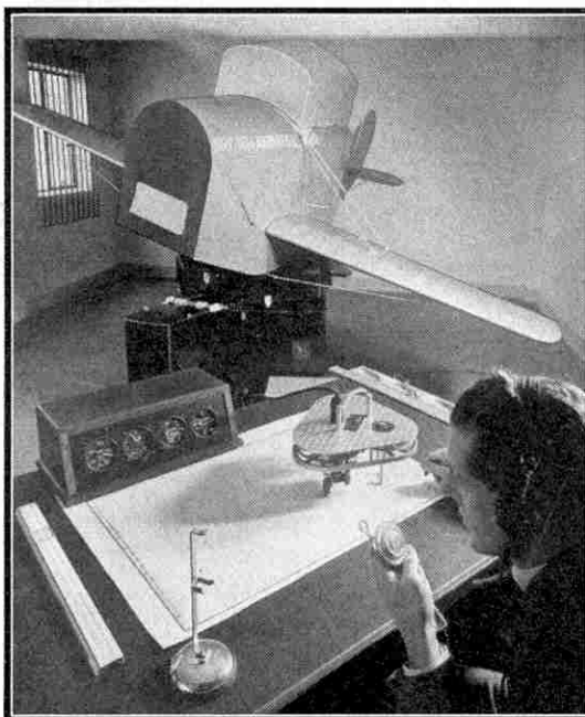
Instrument flying on the Link Trainer. The instructor is telling a pilot that visibility at the terminal aerodrome is so bad that a "blind approach" is necessary.
