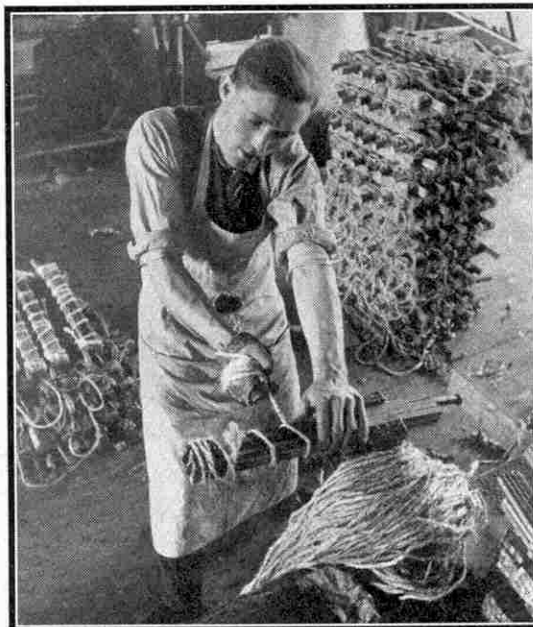
Glueing slips of four canes each together to form a bat handle. The wrapping keeps the canes pressed tightly together until the glue dries. There are four slips, or 16 canes, in each handle.
