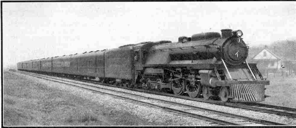
The " Abraham Lincoln " hauled by a steam locomotive. The engine is the 4-4-4 " Lady Baltimore ," which is seen also on our cover. This locomotive incorporates certain features of G.W.R. practice.
