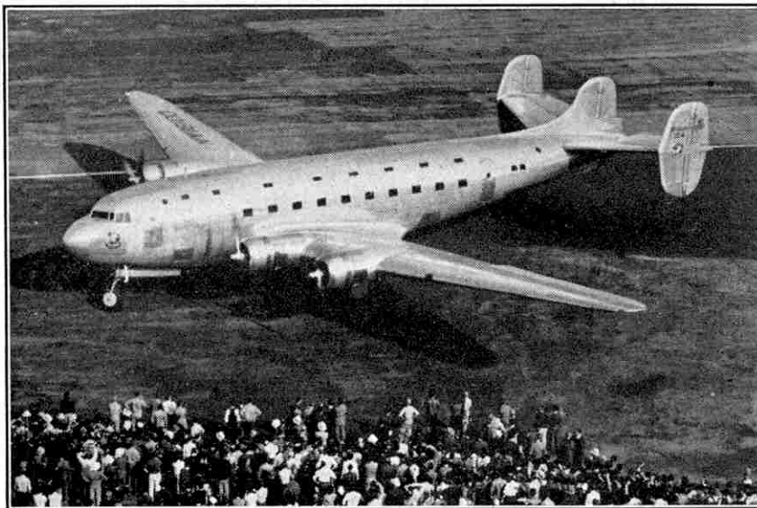
The first Douglas DC-4 about to take off for its maiden flight, the first of a long series of test flights. This huge four-engined air liner has a wing span of 138 ft., and a range of 2,200 miles, and will carry 42 passengers and a crew of five. Photograph by courtesy of the Douglas Aircraft Company, Inc., U.S.A.
