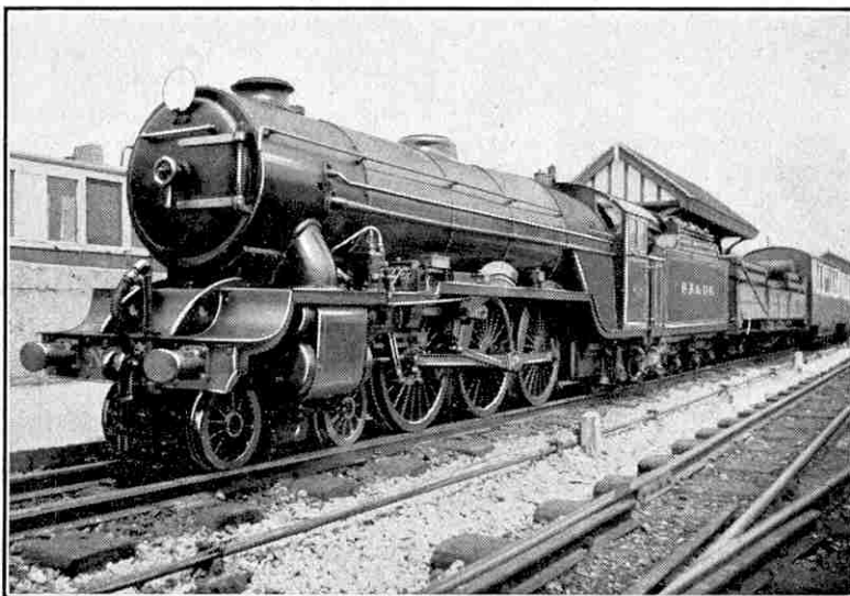
"Green Goddess," one of the 4-6-2 express engines of the 15 in. gauge Romney, Hythe and Dymchurch Railway. The resemblance to the full-size Gresley "Pacifics" of the L.N.E.R. is a striking feature.
