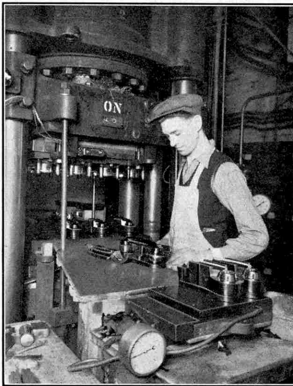
Moulding hand-sets in a 350-ton press, in which four are made at once. The illustrations to this article are reproduced by courtesy of the Telephone Manufacturing Co. Ltd., London.
