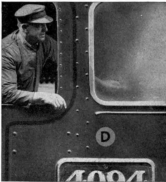
The classification disc and letter on a G.W.R. engine. From "G.W.R. Engines," reviewed on this page.
