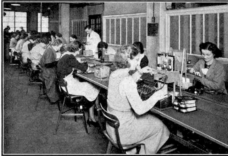
The conveyor on which bell-sets are assembled, stage by stage. Soldering work is being carried out in the centre, and the sets are being tested on the right on either side.
