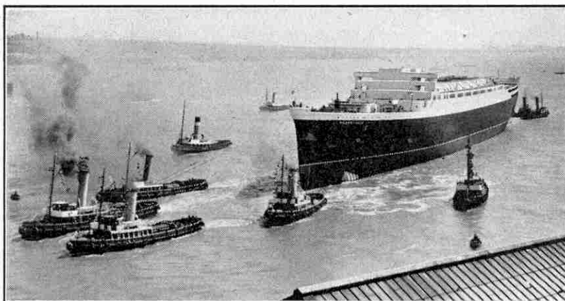
The "Mauretania" in the water, with eight tugs guiding her to the fitting-out basin. The width of the Mersey at this point allowed the vessel to be launched freely, without drag chains to check her run.
