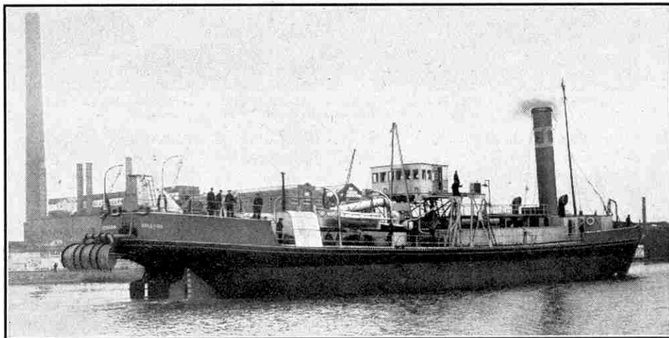
The steam suction dredger "Severn." It is the finest of the large and powerful vessels employed at the Port of Bristol in keeping the River Severn clear of silt. Photograph by courtesy of W. Symons and Co. Ltd., Renfrew.
