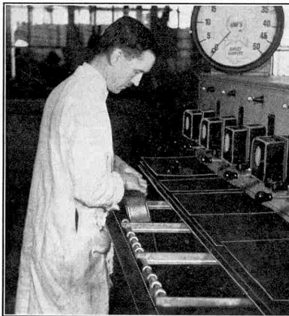
A container holding a wax disc being placed in an electrolytic bath, in which it is slowly revolved during plating operations.
