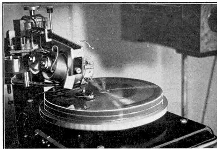
Recording in progress. The threads cut from the wax disc by the sapphire are drawn off by a suction device.
