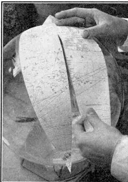
Fitting two of the 12 map sections together. The greatest accuracy is necessary in this work.
