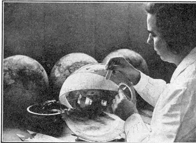
Gluing a map section on a glass globe. There are 12 sections to each globe, and they are illuminated by an electric lamp placed inside it.
