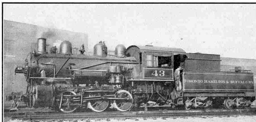
A 0-6-0 shunting or "switching" locomotive of the Toronto, Hamilton and Buffalo Railway. The New York Central System and the C.P.R. have joint interests in this line. Photograph by H. McMichael, Waterford, Ontario.
