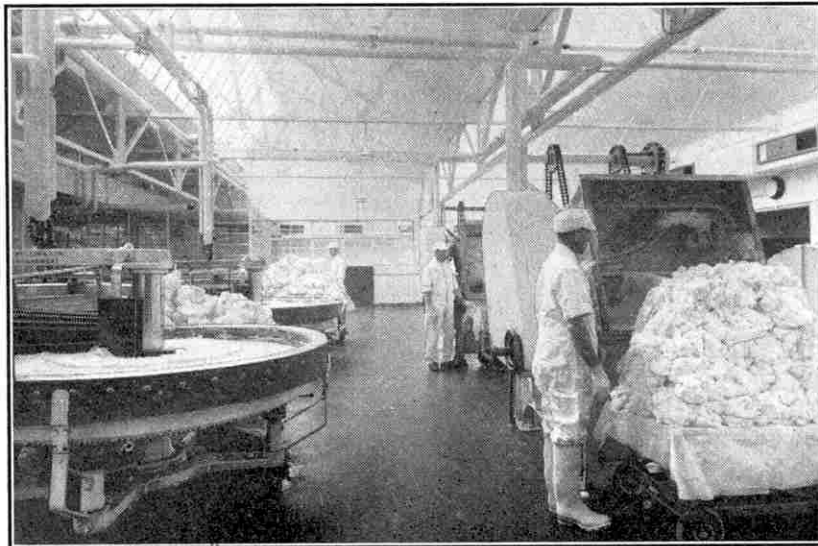
The big circular tables on which butter is passed under rollers that make it smooth and consistent and remove surplus water. The necessary salt also is added in this room. The illustrations in this article are reproduced by courtesy of Wilts. United Dairies Ltd., Yonder Hill, Somerset.
