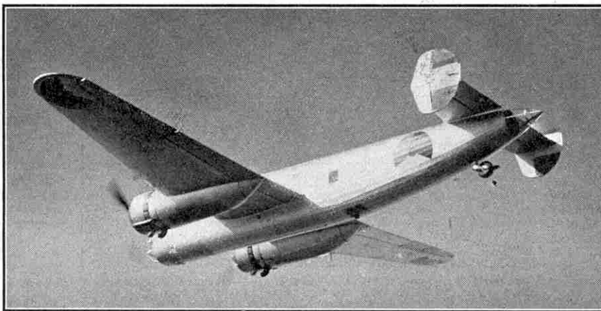
A T.5 long-range bomber in the air. This view shows the middle wing form of construction and the conical turret that forms the pointed stern.
