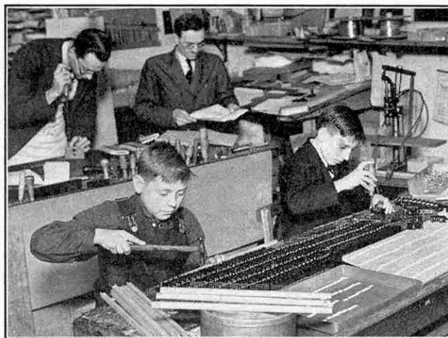
Early stages in organ making. At work on double contact breakers for use with the stop keys used on many church and concert organs.
