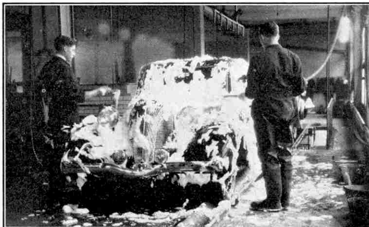
The snowstorm effect on this car is produced by spraying soap foam all over the bodywork in order to loosen grease and dirt.
