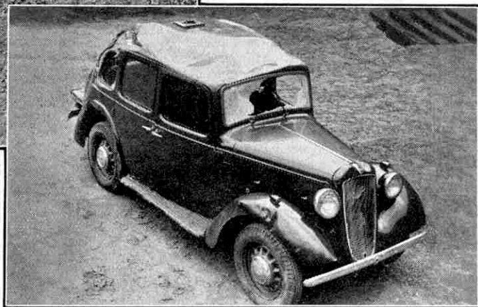
From left to right are shown three stages in the drastic test of a motor car described in this article. The car rolled over several times and crashed into a road, finishing battered but with engine and mechanism undamaged. Photographs by courtesy of Austin Motors Ltd., Birmingham.
