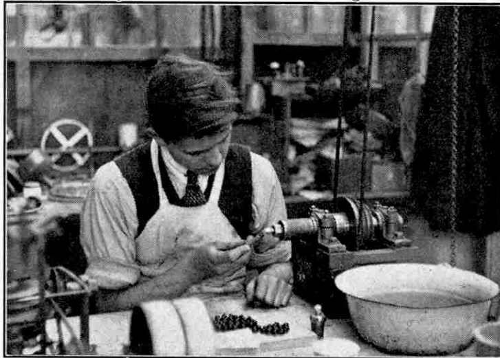
Hand polishing tiny lenses for use in photomicrography. The polishing is carried out with rouge or putty powder, which cuts off the uneven parts.
