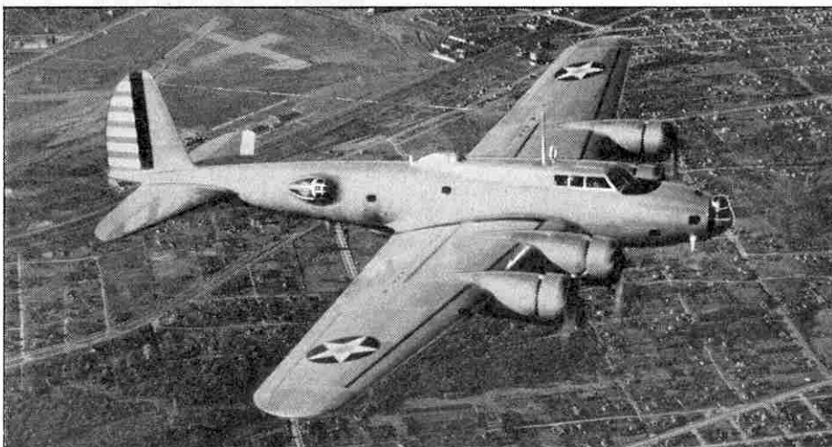
The first photograph of the new Boeing YB-17A "Flying Fortress" Bomber. It carries a crew of seven to nine men, and is fitted with special engine superchargers for operation at very high altitudes. Photograph reproduced by courtesy of the Boeing Aircraft Company, U.S.A.
