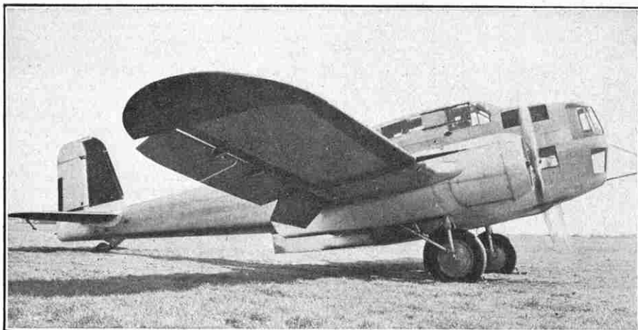
The Breguet 462B-4, a modern French twin-engined fighter and bomber. It is armed with three guns and carries a heavy load of bombs inside the fuselage.
