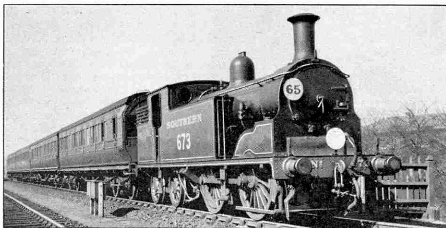
Former L.S.W.R. M7 class 0-4-4 tank engine, No. 673, on the West London Extension Railway at Battersea. Photograph by W. P. Conolly, London S.W.11.
