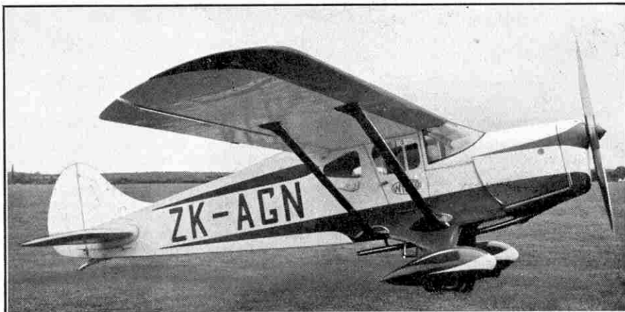
This "Wicko" 2-seater cabin monoplane was the first of a series delivered to New Zealand last year, and now in use there as trainers. Photograph by courtesy of Foster, Wikner Aircraft Co. Ltd.
