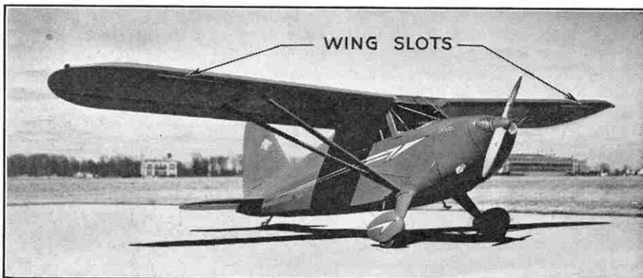
The Stinson "105" described on this page. A special feature of this machine is the use of built-in wing slots. Photograph by courtesy of the Stinson Aircraft Division, U.S.A.
