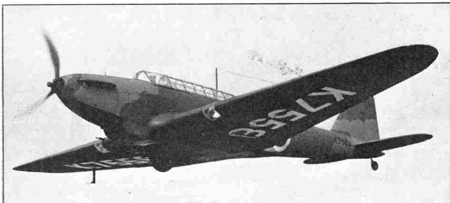
A striking view of the Fairey "Battle." The barrel of the fixed Browning gun can be seen near the landing light in the starboard wing. Photograph by courtesy of "Flight."
