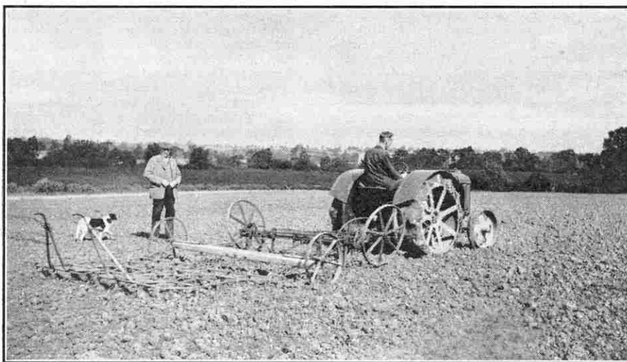
A tractor hauling a set of harrows and a slicer. Normally six horses would be needed for this work.
