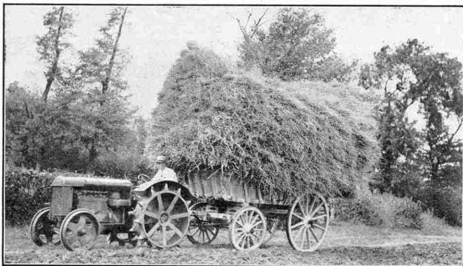
An ordinary farm wagon fitted with a drawbar instead of shafts so that it can be hauled by a tractor.
