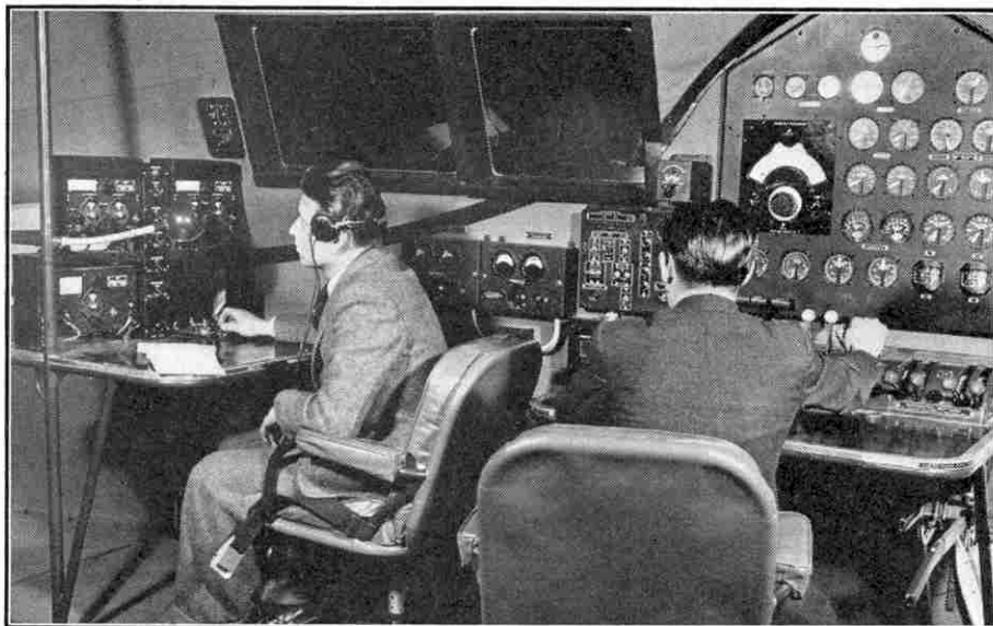
The flight engineer's and radio officer's stations in the control room of the new Boeing 314. An article describing these flying boats appears on page 470 of this issue.
