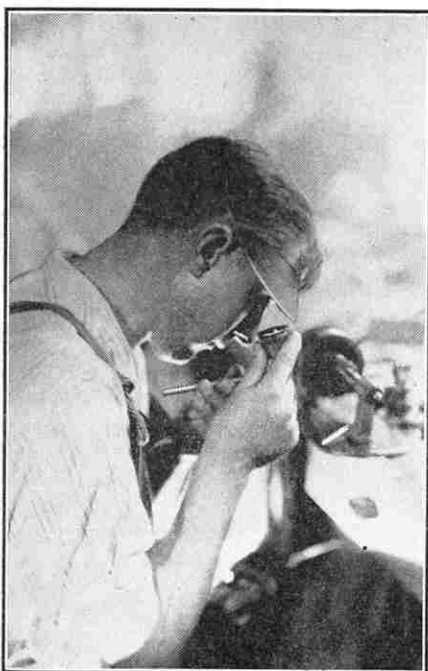
Grinding a gold nib to finish the point.
