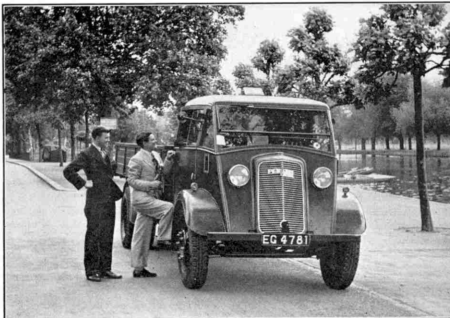
The Commer "Q" type Diesel-engined lorry, which has been designed round the Diesel engine.
