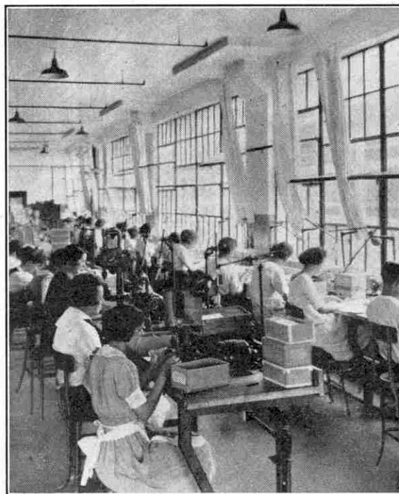
Fitting clip caps in the assembly of fountain pens.
