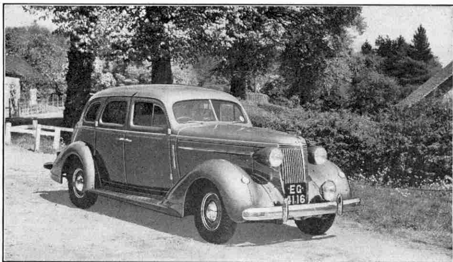
The Nash "Ambassador," in which a Perkins Diesel engine is fitted. The car's maximum speed is 90 m.p.h. The illustrations to this article are reproduced by courtesy of F. Perkins Ltd., Peterborough.
