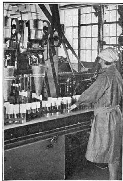
Weighing cocoa automatically into tins.
