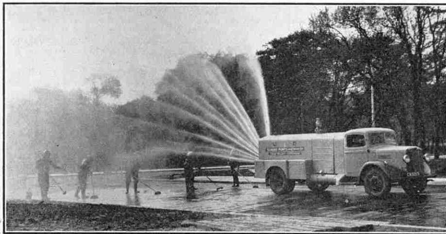
A Morris-Commercial Sigmund decontamination lorry in action. A description of the lorry is given on the previous page. Photograph reproduced by courtesy of Sigmund Pumps (Great Britain) Ltd., Gateshead-on-Tyne.
