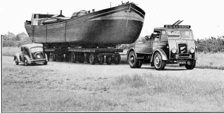
A big transport job. The illustration shows a Foden Diesel hauling a 70-ft. boat weighing 43 tons. Photograph reproduced by courtesy of Fodens Ltd., Sandbach.
