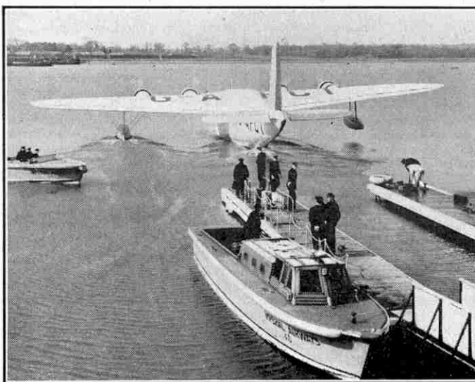
The flying boat "Champion" being warped into the twin pontoons at Berth 108, Southampton. Photograph reproduced by courtesy of Imperial Airways Limited.
