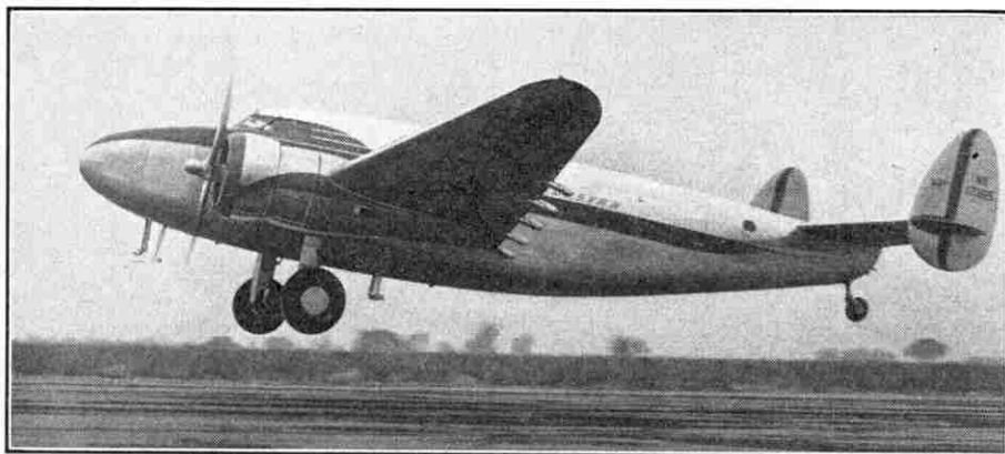
The "Lodestar," the latest Lockheed commercial transport. It is a middle wing monoplane seating 17 passengers. The photographs on this page are reproduced by courtesy of the Lockheed Aircraft Corporation, U.S.A.
