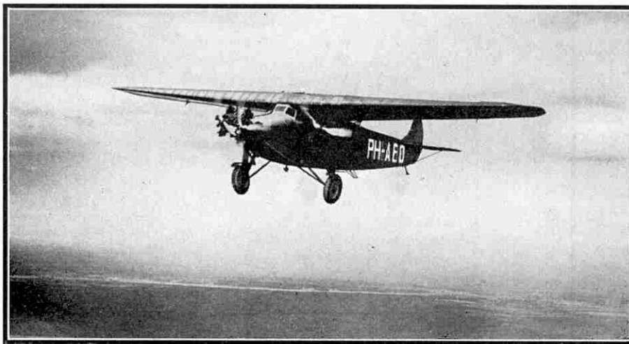
A Fokker F.VIIb-3m triple-engine monoplane in operation in 1932 on one of the air services of Royal Dutch Air Lines, by whose courtesy this photograph is reproduced.
