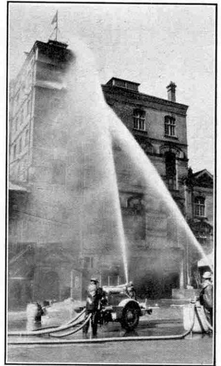
A Scammell trailer type fire-fighter in action. A description of the trailer appears on this page.
