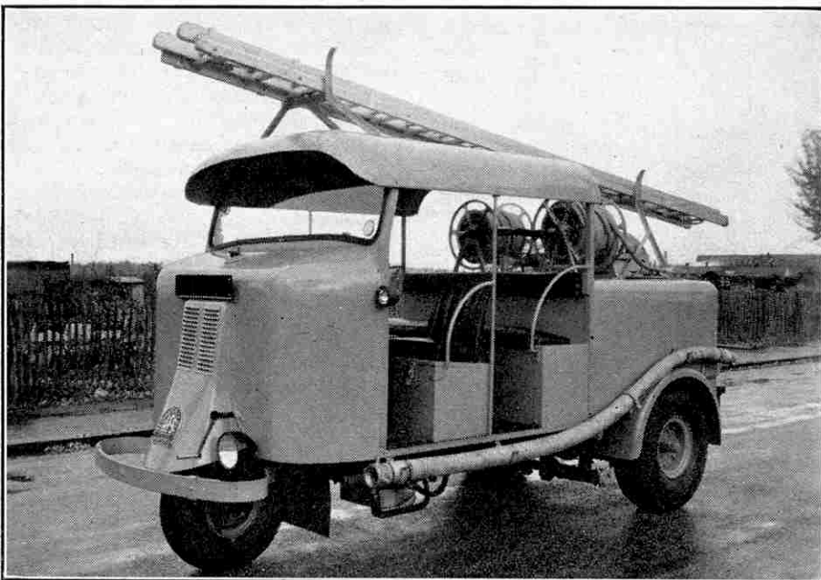
A novel Scammell fire engine with a three-wheeler chassis of the mechanical-horse type. This illustration and the one above are reproduced by courtesy of Scammell Lorries Ltd., Watford.
