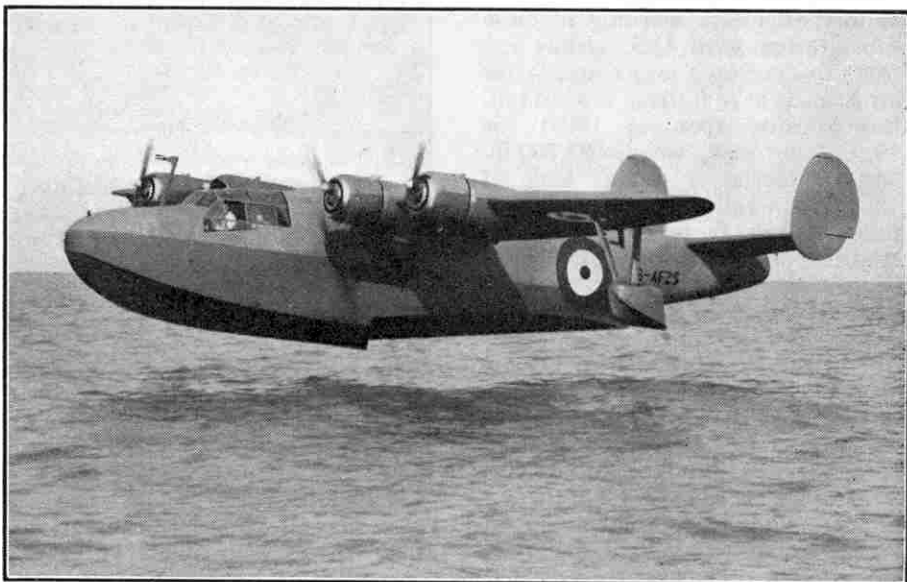
The 50 ft.-span scale model flying boat built by Saunders-Roe Ltd., Cowes, to whom we are indebted for this photograph. The boat can carry a passenger in addition to the pilot.
