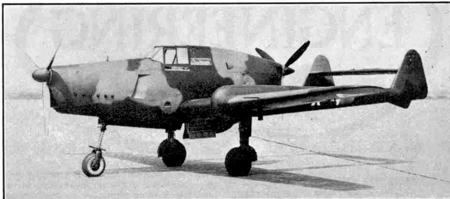
A Fokker D 23 single-seater Fighter. It has two 540 h.p. Walter "Sagitta" engines, mounted one at each end of the short fuselage, and can attain a top speed of about 385 m.p.h. Photograph by J. I. Dorgelo, Jr., Holland.
