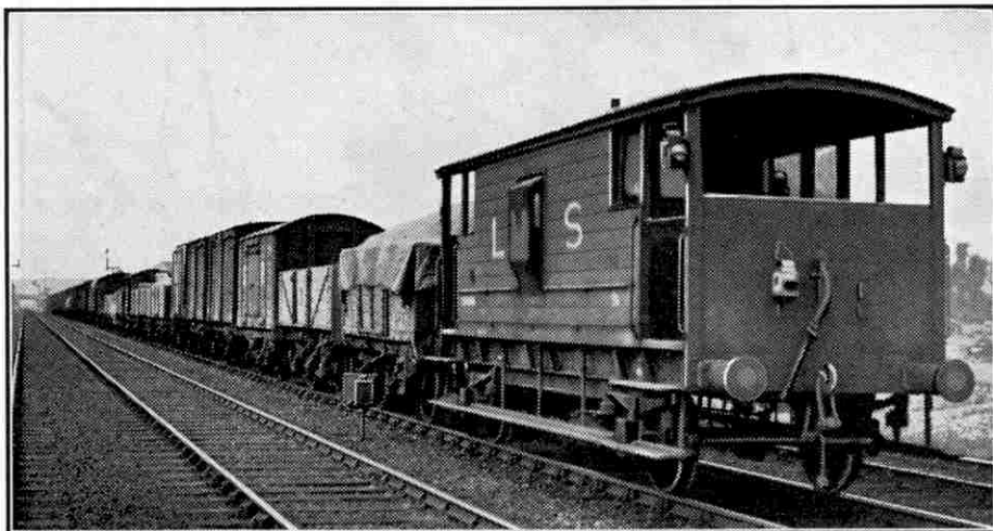
Tail-end view of an L.M.S. fitted freight train. This is the type of van in which the author rode from Manchester to Glasgow. The illustrations on this page are from photographs by E. R. Wethersett
