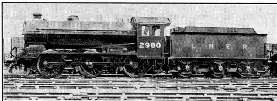
L.N.E.R. standard "J39" class 0-6-0 locomotive, which is suitable for general goods work and for certain types of passenger work. Photograph by W. H. Whitworth.
