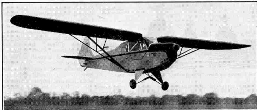
A Luton "Major" two-seater monoplane. The wings can be folded back, enabling the machine to be stowed in a small hangar. Photograph by courtesy of "Flight."
