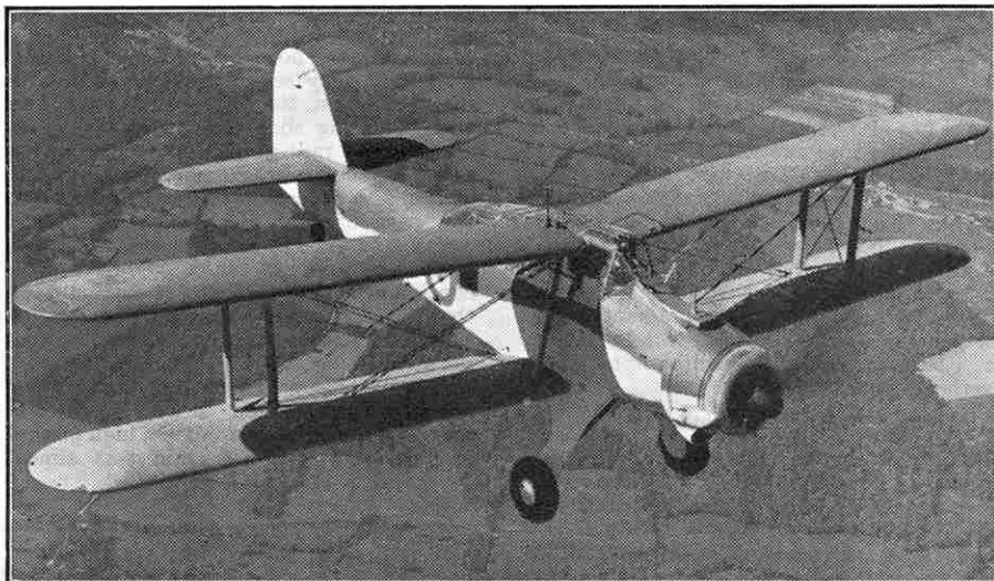
The Fairey "Albacore," which can be used for dive-bombing, torpedo dropping, reconnaissance, and fleet spotting. It is an equal-span biplane. Photographs by courtesy of the Fairey Aviation Co. Ltd.
