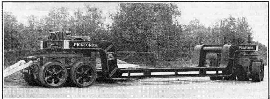
A 16-wheeler girder frame trailer designed for carrying loads up to 80 tons. It was built by Cranes (Dereham) Ltd., to whom we are indebted for our illustration.
