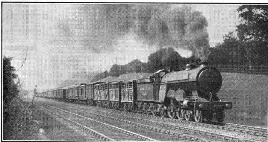
This engine has its boiler mountings and cab altered to suit the loading gauge of the Northern Area of the L.N.E.R. Photograph by W. H. Whitworth.
