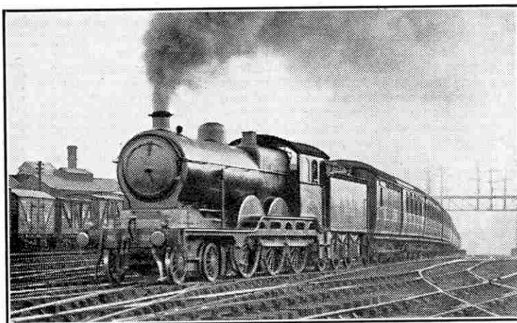
Continental Express topping Bethnal Green bank. Unrebuilt "B12" 4-6-0 No. 8533. Photograph by F. R. Hebron.
