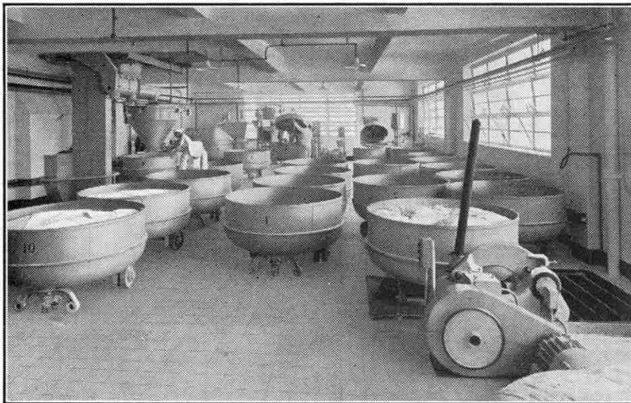
The dough room. The machine that blends and weighs the flour is on the left, and the dough mixing machines are at the far end of the room. On the right is a tipping machine, which tilts up the bowl to empty the risen dough on to a grid over the hopper leading to the dividing machines.
