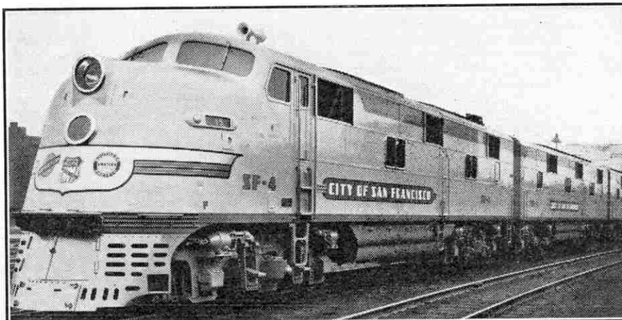
A power plant on wheels; one of the two new triple-unit 6000 h.p. Diesel-electric streamliners introduced for haulage of 18-car trains between Chicago and the Pacific Coast. Illustrations by courtesy of the Union Pacific Railroad.
