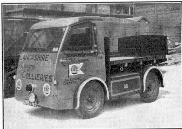
A neat electrically-driven coal lorry. It is supplied with current from storage batteries, and is a product of Metropolitan-Vickers Electrical Co. Ltd., Manchester, to whom we are indebted for our illustration.
