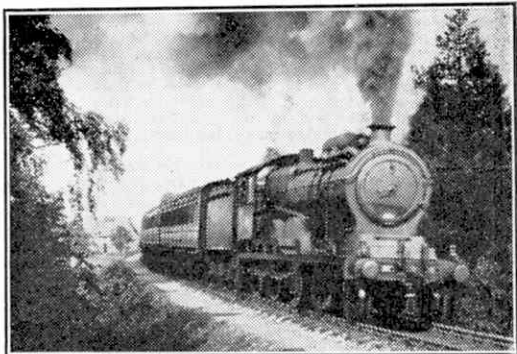
An Inverness-Aberdeen express, on the G.N.S. section of the L.N.E.R., climbing a bank of 1 in 60. The engine is one of the former G.E. "1500" class. Photograph by W. Watt, Lhanbryde, Morayshire.
