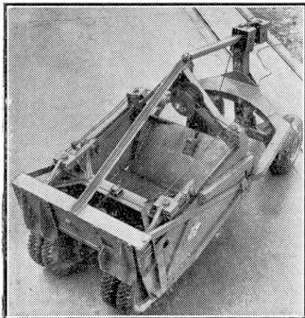
Fig. 1. Blaw-Knox Scraper, showing the cable operation. The photographs in this article are by courtesy of Blaw-Knox Limited, London.
