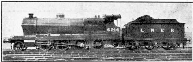
L.N.E.R. 2-8-0 No. 6214, one of the Class "04" engines of former G.C. design. Photograph by courtesy of the L.N.E.R.
