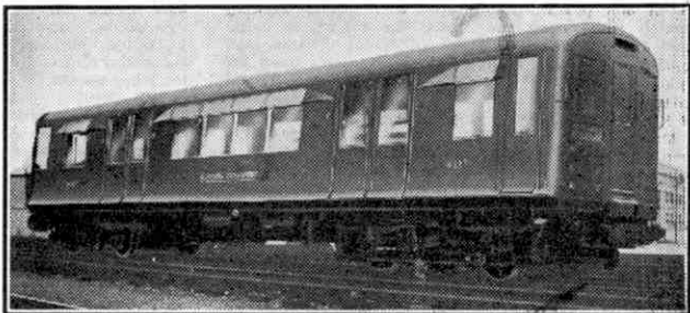
The finished car, numbered 14233, constructed from the remains of two cars severely damaged in an air raid.
