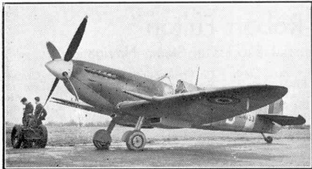
This view of the latest version of the famous "Spitfire" fighter shows the slightly longer nose made necessary by the fitting of the Rolls-Royce "Merlin" 61 engine in this machine. Photograph "The Aeroplane" copyright.
