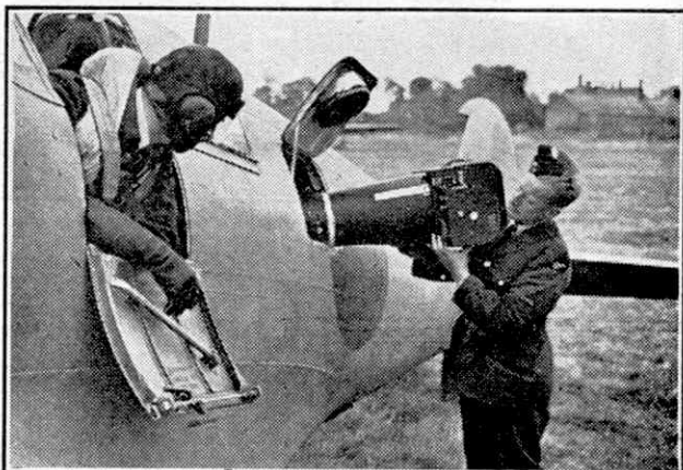
The same airman loading the camera into the "Spitfire." These aircraft carry two of these big cameras set at an angle to one another so that they cover a strip of country on each side of their track, and overlap in the middle. Smaller cameras also are carried.
