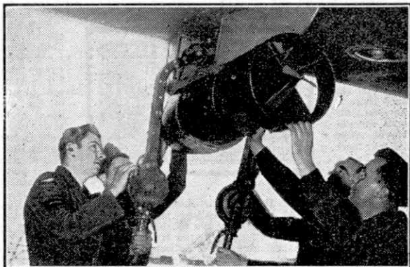
Fitting a 500 lb. bomb to the wing of a "Mosquito." Photograph by courtesy of de Havilland Aircraft Co. Ltd.
