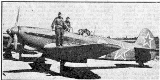
The YAK-9 fighter, shown here, has a top speed of about 390 m.p.h., and is the fastest Russian warplane.
