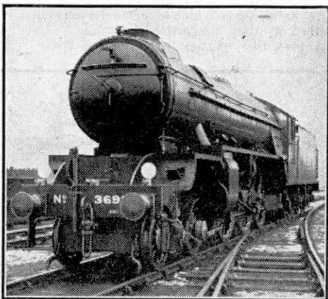
L.N.E.R. "Pacific" No. 3698, of the "A2/1" Class, which has been fitted with electric lights on the front of the engine and rear of the tender, and also in the cab. Photographs by courtesy of the L.N.E.R.
