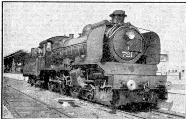
Compound 4-6-0 locomotive No. 721 of Class "7" of the Belgian National Railways. Photograph by C. R. L. Coles.
