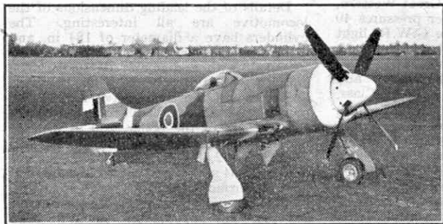
Another view of the "Tempest" II, the engine of which is the Bristol "Centaurus," the most powerful radial engine in service anywhere.
